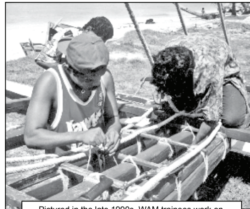
Pictured in the late 1990s, WAM trainees work on lashing intricate parts of a canoe together. Below, trainees are taught how to create a thatched roof on the new Waan Aelon in Majel building next to the Marshall Islands Resort.
